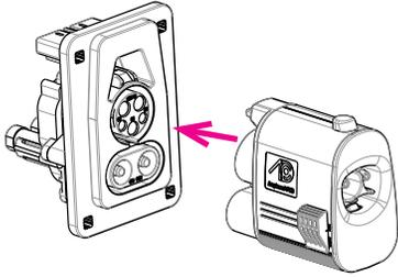
2. Press the NACS J3400 DC Charging cable plug into the NACS end of the adapter until it is fully seated (audible "click").
