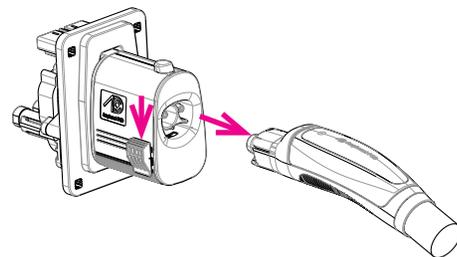
2. Remove the adapter from the vehicle with pressing the CCS1 Unlock Button on the top of the adapter.
