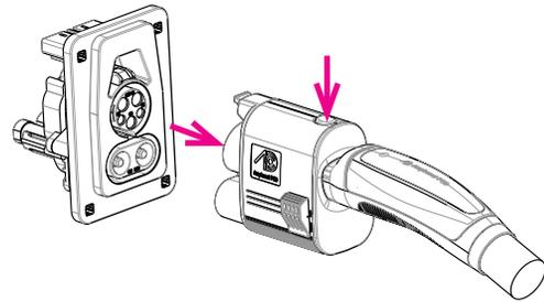
2. Pull the plug out of the adapter with pressing the NACS Unlock Button on the side of the adapter.
